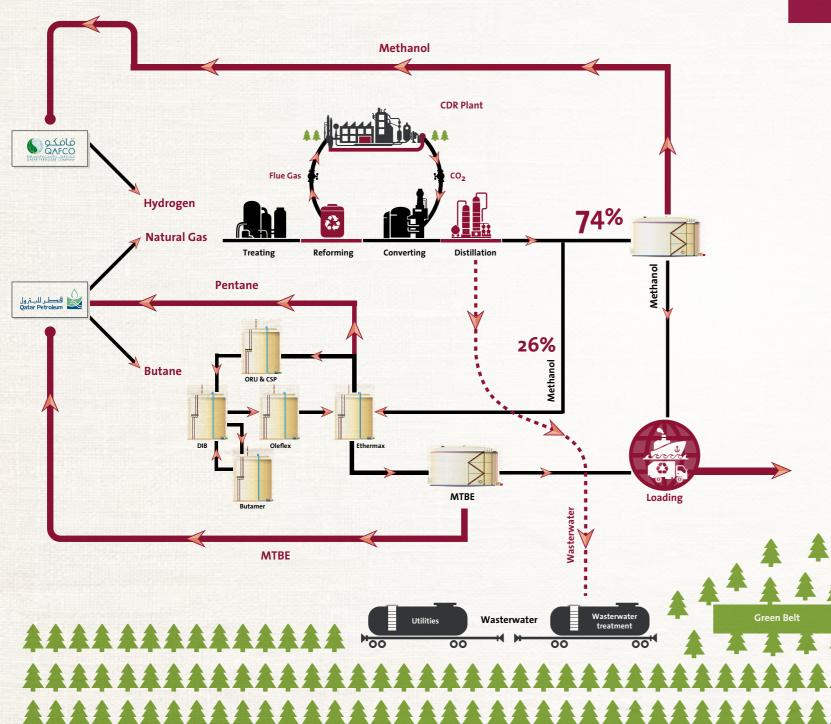
QAFAC is a unique standalone integrated facility (i.e. not connected directly to a refinery), where MTBE production is not situated in an integrated refinery as is typical in other parts of the world.
